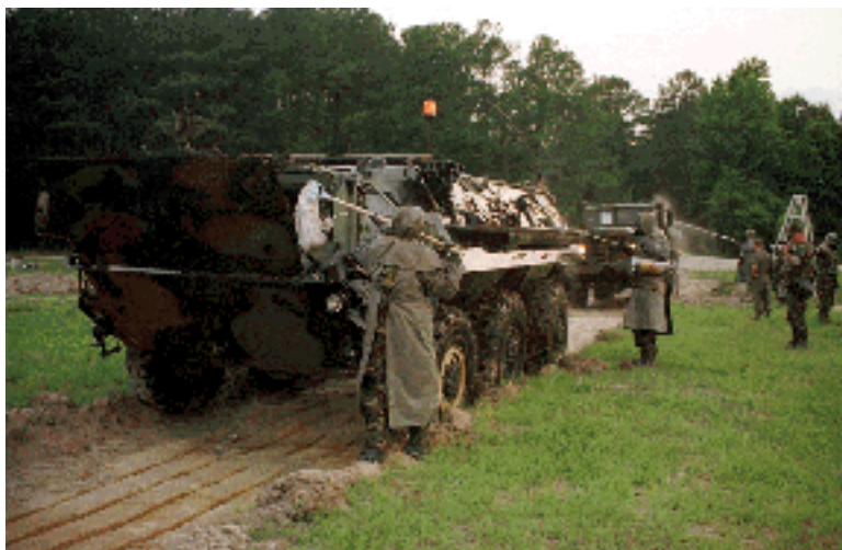
Thorough decontamination is supported by specialized decontamination units and personnel.
